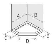
For pentagonal trays, the three measurements shown in the diagram must be taken from the external part of the tray to the wall.
