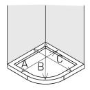
For curved trays, two measurements must be taken, from the external part of the tray to the wall and the diagonal measurement of the tray, as shown in the diagram.
